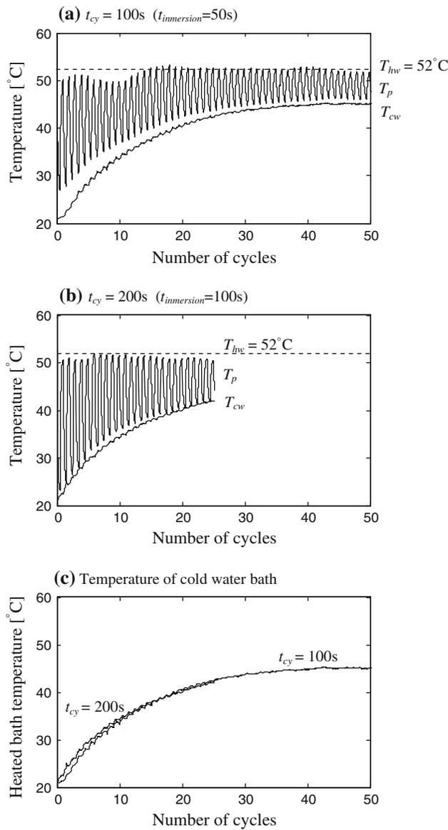
**Fig. 3** Measured heat transfer in two-baths experiments. Temperature evolution with number of cycles for immersion duration  $t_{cy} = 100$  s and 200 s.  $T_p$ : particle temperature.  $T_{hw}$ : constant hot water bath temperature  $52^\circ\text{C}$ .  $T_{cw}$ : cold water bath temperature
