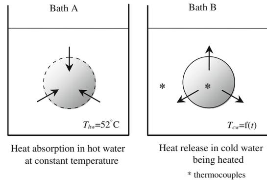
**Fig. 2** Heat transfer by repeatedly moving a heated particle from the constant temperature hot water bath "A" into a cold water bath "B" of finite mass
