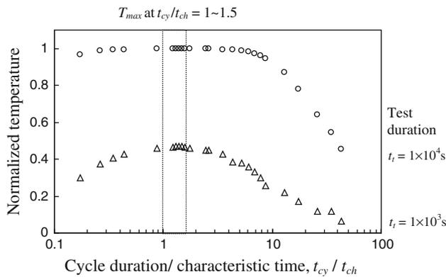
**Fig. 5** Predicted temperature of the water bath at selected times for different cycle durations  $t_{cy}$ . The maximum temperature is obtained when  $t_{cy}/t_{ch}$  is  $1 \sim 1.5$ , where the characteristic time  $t_{ch} = 23$  s. The normalized temperature in y-axis represents  $(T_{predicted} - T_{cw}) / (T_{hw} - T_{cw})$
