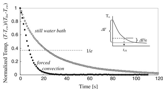
**Fig. 1** Temperature change in a particle ( $r_p = 0.0127$  m) when it is suddenly submerged in a large cold water bath. The insert shows the definition of the characteristic time  $t_{ch}$ . Data shown for cooling in still water and in stirred water
