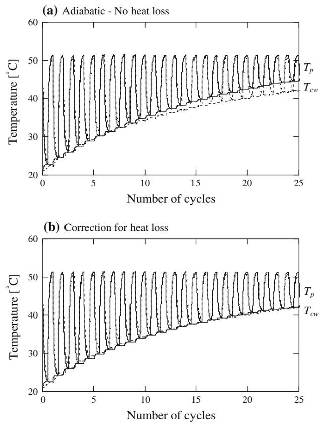
**Fig. 4** Experimental data (dotted lines) and numerical prediction (solid lines) corresponding to the particle and the water bath temperature evolution—Cycle duration  $t_{cy} = 200$  s. Numerical predictions in each frame assume: **a** adiabatic conditions—the overestimated bath temperature increases with time; and **b** heat loss to the surroundings (fitting value:  $\Psi = 0.05\text{W }^\circ\text{C}^{-1}$ ). Note:  $T_p$  particle temperature;  $T_{cw}$  cold water bath temperature
