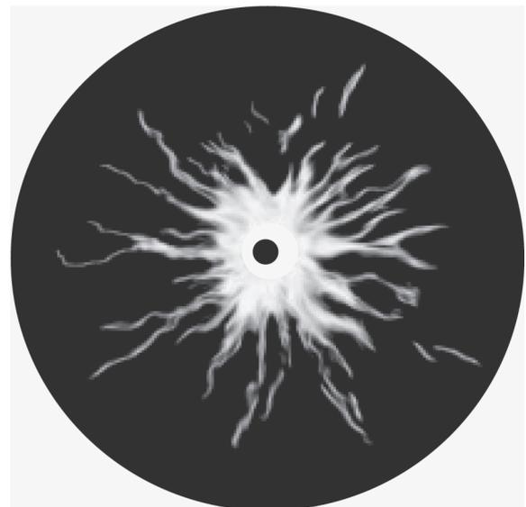
Fig. 8—Nonlinear particle-entrained radial fluid flow in porous networks. Localized flushing and finger formation in a porous medium containing small mobile particles, where  $d_o/d_p > \delta_{\max}$ . Black represents the fine-bearing sediment, and white shows the fine-depleted zones.
