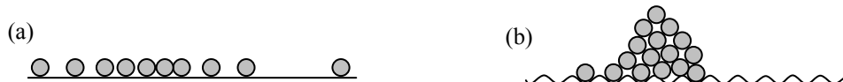
Figure 25. Boundary conditions and friction. Smooth spherical particles do not form a granular pile on a polished flat surface (a), but readily form the pile on a corrugated surface (b).
