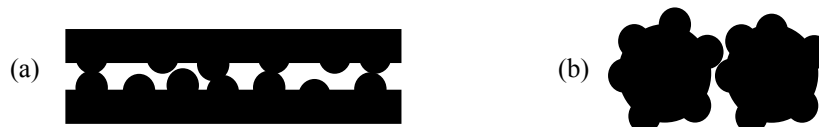
Figure 1. Effect of surface topography. (a) Large surfaces: the true area of contact is independent of surface topography when contacts deform either elastically (exponential height distribution) or plastically. (b) Grains: the same scale of surface topography may cause interlocking between grains.
