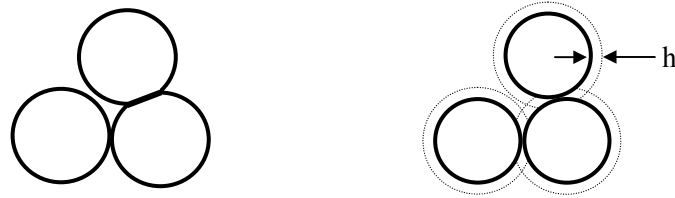
Figure 13. Contact forces and contact deformability - Degradation threshold strain. (a) Large particles: Hertzian deformation. (b) Small particles: electrical interaction.
