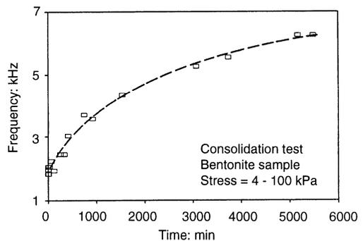
Fig. 11. Variation of the natural frequency of a bender element installation during the consolidation of a very soft bentonite, from  $\sigma_v' = 4$  kPa to  $\sigma_v' = 100$  kPa
