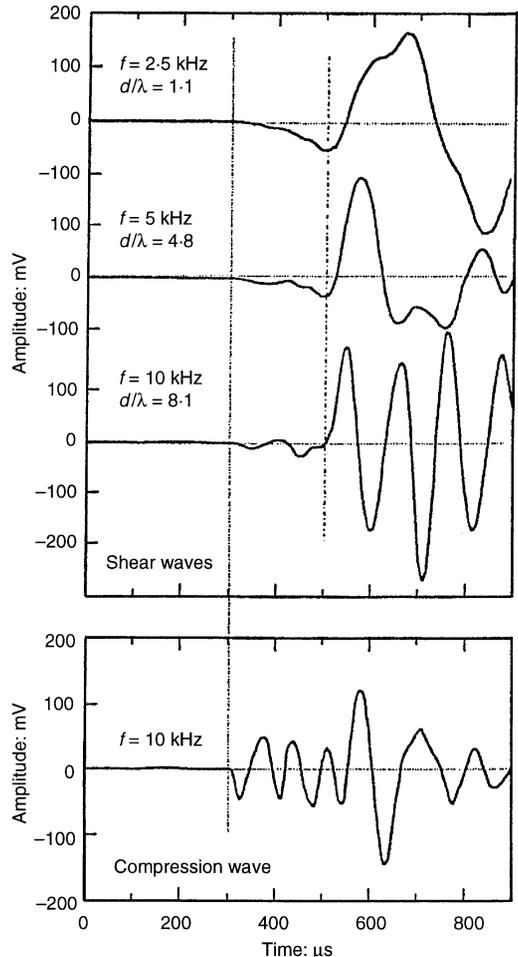
Fig. 12. Shear and compression waves received by bender elements in tests on dry Ticino sand (after Brignoli & Gotti, 1992)
