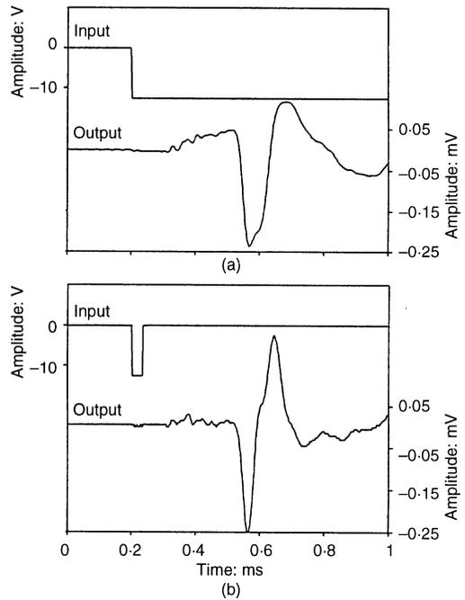
**Fig. 9.** Typical response for a bender element with deteriorated insulation in a saturated silty soil, subjected to a step and a short pulse excitation ( $\sigma_v' = 40$  kPa)
