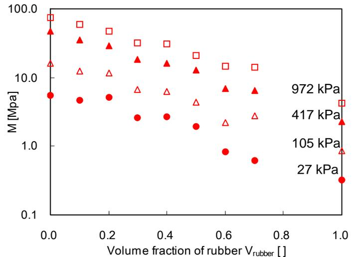
Fig. 5 Constrained modulus in sand-rubber mixtures versus applied vertical stress.
