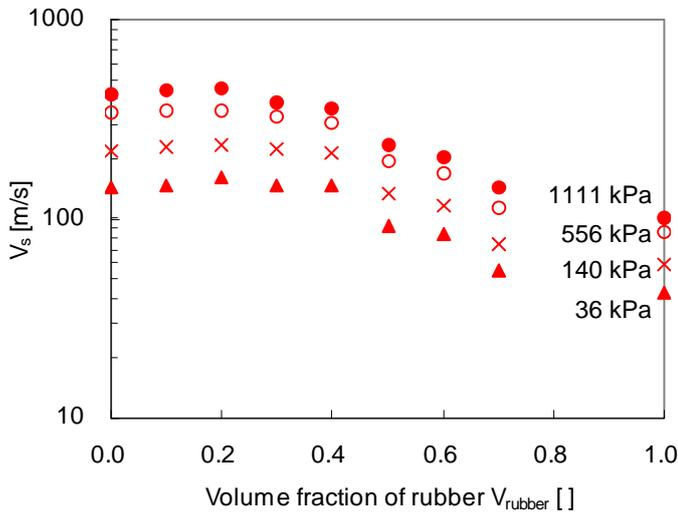
Fig. 6 Shear wave velocity in sand-rubber mixtures
