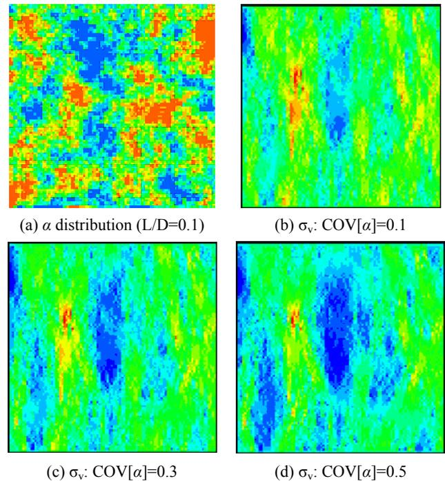
Fig. 3 Vertical stress focusing: Variance leads to arching and load transfer through stiffer vertical columns
