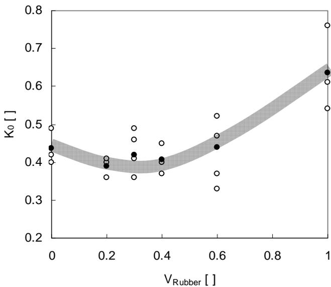
Fig. 7  $K_0$  values in the soil-rubber mixtures (black dots are the average values)
