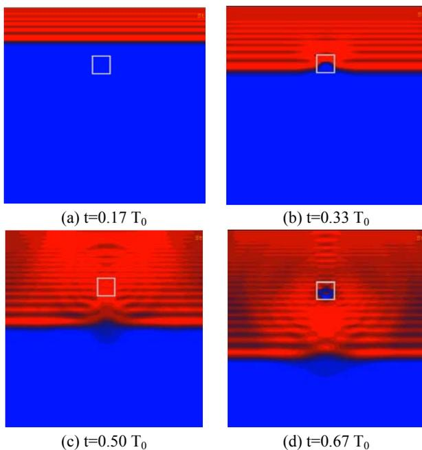
Fig. 4 Plane S-wave propagation in a medium with a low velocity inclusion. Notation:  $T_0 = L/V_{s0}$ , the inclusion size  $D \approx 1.6\lambda$ ,  $t =$  time.
